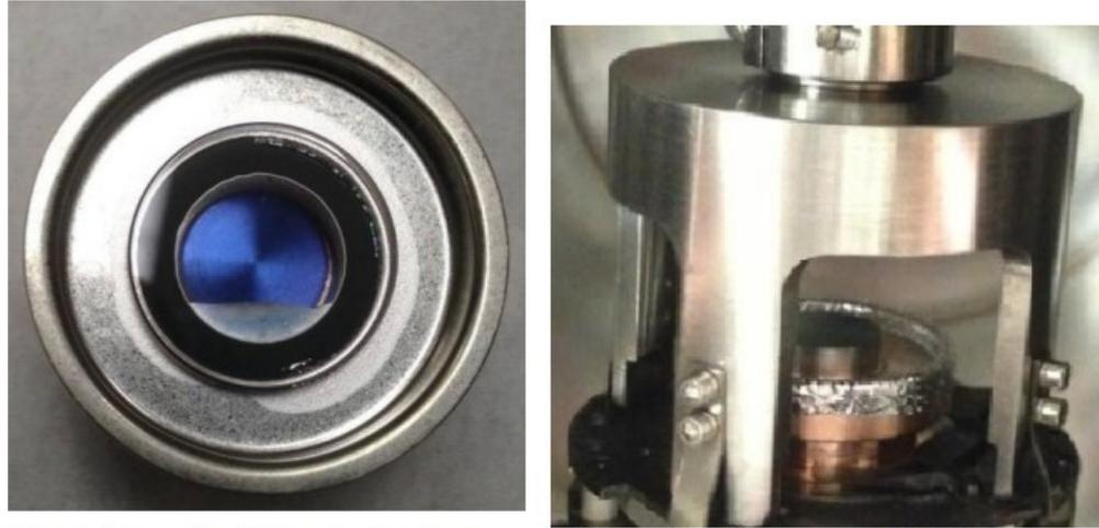
Capsule-sealed Photonis photocathode with the cap on (left) and removed (right)
